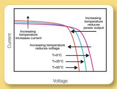
Since PV modules produce their highest voltage at the lowest temperatures, this voltage determines the minimum voltage ratings required for the modules and associated dc circuit components [NEC 690.7]. For crystalline silicon PV modules, the maximum voltage for PV arrays
