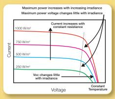
Therefore, doubling the solar irradiance on the surface of the array doubles the current and maximum power output (assuming constant temperature). Changing irradiance has a smaller effect on voltage, mainly at lower irradiance levels. Because voltage varies little with changing irradiance levels over 200 W/m2, PV devices are well-suited for battery charging applications. See Figure 5.
