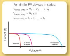
Connecting PV modules in series with dissimilar current ratings results in loss of power, similar in effect to partially shading an array, or having parts of a series source circuit located on surfaces facing different directions and receiving different levels of solar irradiance. The resultant
