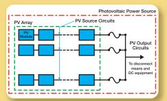
A string is a series connection of PV devices. PV cells or modules are configured electrically in series by connecting the negative terminal of one device to the positive terminal of the next device, and so on. For the series connection of similar PV modules, the voltages add and the resulting string voltage is the sum of the individual module voltages. The resulting string current output remains the same as the current output of an individual module. See Figure 8 & Figure 9.
