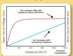
The short-circuit current (lsc), maximum power current (lmp), and maximum power (Pmp) at one condition of solar irradiance may be translated to estimate the value of these parameters at another irradiance level:
